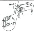
Step 1: Secure right leg (A) with washer (D) Step 2: Secure left leg (A) with washer (D) and and screws (E) by using allen wrench (G). Do screws (E) by using allen wrench (G). not fully tighen now.
