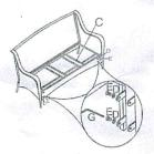
Step 3: Secure seat panel (C) to assembled sofa arms (A1.A2) with 4 washer (D) and 4 screws (E) by using allen wrech (G). Do not fully tighen now.
