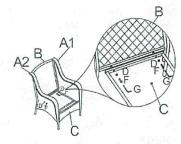
Step 4: Secure seat panel (C) to assembled sofa back (B) with 2 washer (D) and 2 screws (F) by using allen wrench (G), verify the alignment and adjust, fully tighten all the screws now.
