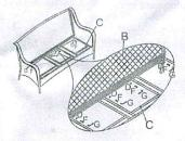
Step 4: Secure seat panel (C) to assembled sofa back (B) with 4 washer (D) and 4 screws (F) by using allen wrench (G), verify the alignment and adjust, fully tighten all the screws now.
