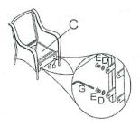
Step 3: Secure seat panel (C) to assembled sofa arms (A1.A2) with 4 washer (D) and 4 screws (E) by using allen wrech (G). Do not fully tighen now.
